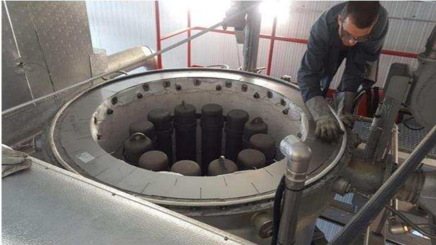
Figure 9 Combustion chamber with improved seal and repaired insulation
